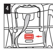
From bottom of seat, locate buckle's metal clip.
